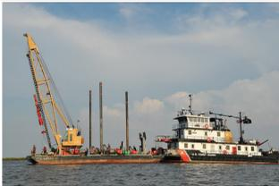
WLICs construct, repair, and maintain fixed aids to navigation within inland waterways. The WLIC is the only Coast Guard platform with the capability to drive and remove piles, erect towers, and effect major structural repairs.
