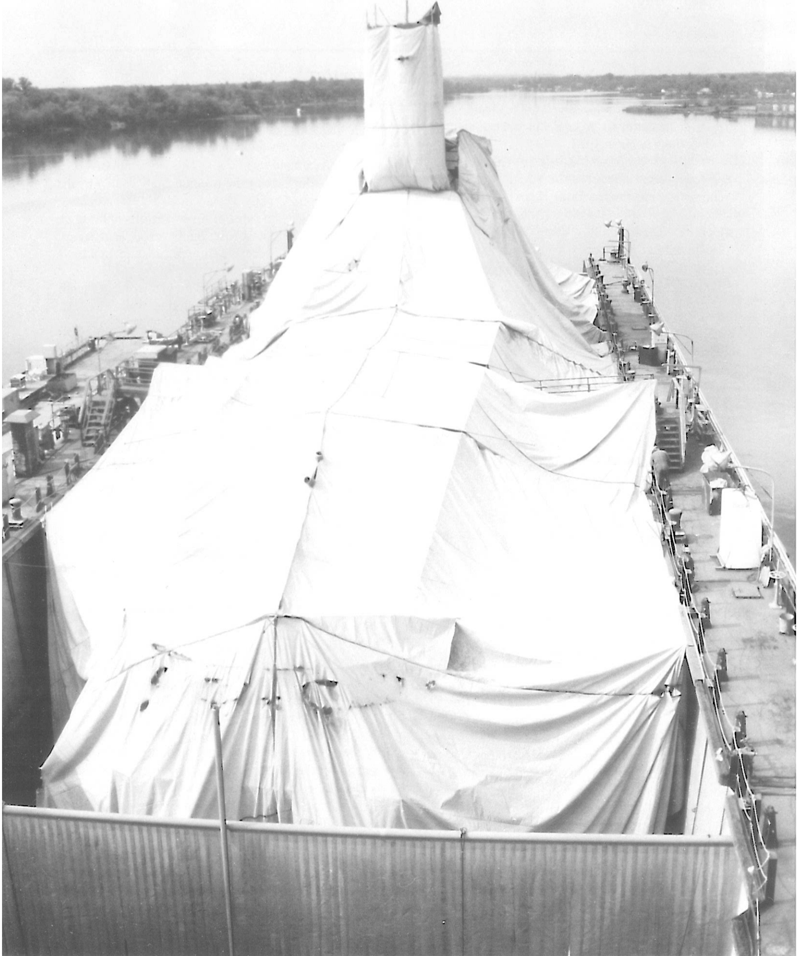
Under The Big Top! The Cutter VALIANT is pictured under the shroud while in drydock undergoing 210' Major Maintenance Availability at the YARD.
