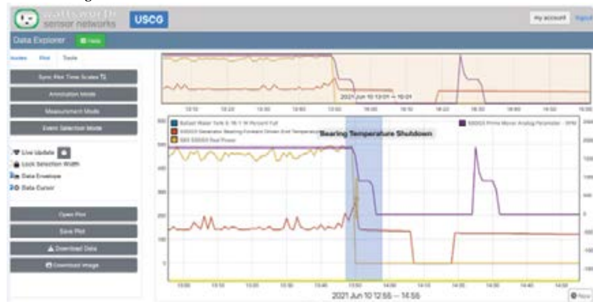
Figure 1: Wattsworth Sensor Networks Monitoring a Bearing Temperature Shutdown from SSDG3
