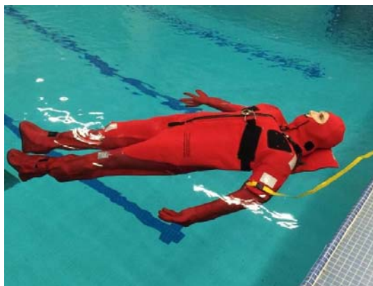
Figure 5. Weighted mannequin/immersion suit flotation trial.
